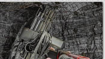
The MBU Anchor Installation Unit is a fully mechanized anchor handling unit with high productivity and a carousel that can be loaded with up to 10 bolts and can handle anchor lengths in the range of 1.5 to 2.4 meters.
