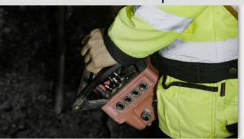
Remote control electric proportional hydraulic intelligent control system, no blind spots in the field of vision during operation, personnel stay away from dangerous places, safe and reliable; Visual adjustment of operation parameters, which can be pre designed to flexibly respond to different working conditions.
