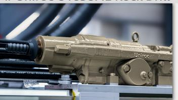
Our self-developed rock drill U1838ME is specially equipped with a secondary buffer system, which greatlyextends the service life of the hydraulic rock drill. It is also equipped with advanced frequency conversion system at all levels, which enables it to flexibly cope with a wide range of different levels of surrounding rock conditions, completely solving the limitation of traditional rock drills that are difficult to be used for multiple purposes.
