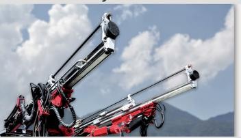
Standard double-layer feed configuration, adaptable to flexible matching of drill rods with different lengths ranging from 2500mm to 4305mm. Other specifications of feed can be optionally configured to flexibly meet the requirements of section excavation, while also meeting the needs of medium-sized section excavation hole operations and anchor hole construction.
