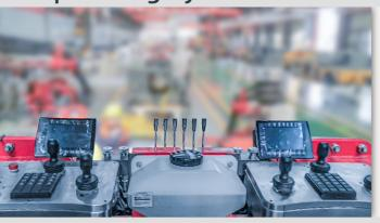
Flexible proportional configuration of rock drilling parameters, setting up a "multi-level automatic matching system for rock drilling parameters" to achieve accurate matching of various surrounding rocks and maximize drilling efficiency; Integrated electrical handle control, one click automatic rock drilling with rock drilling handle.
